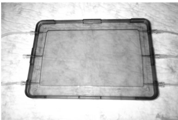
Fig. 1. A gas-permeable polycarbonate cassette with input and output tubing.
